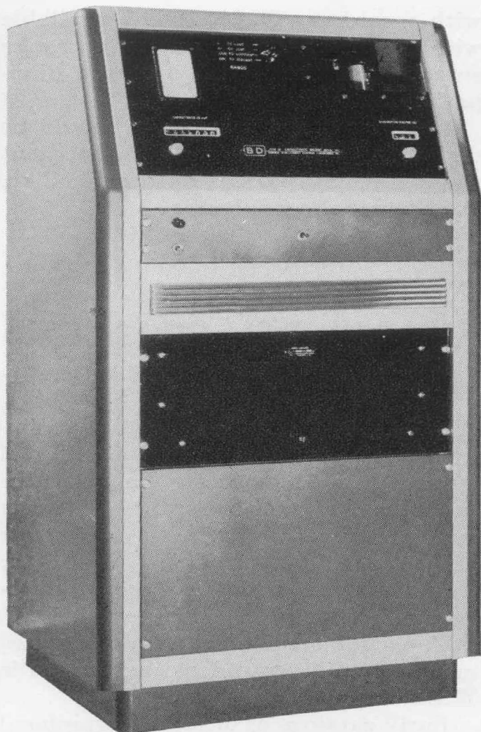
Figure 2. View of the complete bridge assembly.
